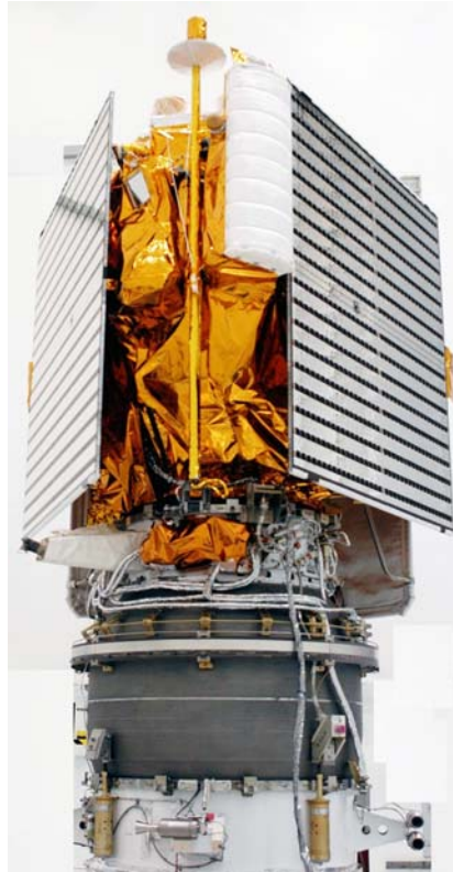
Figure 7. MESSENGER Spacecraft with Solar Panels in Launch Configuration
