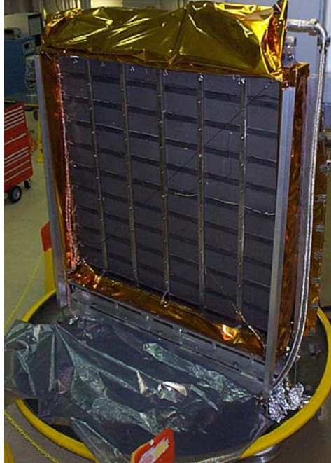
Figure 6. H-Box Used for High-temperature Tests of the Solar Panels
