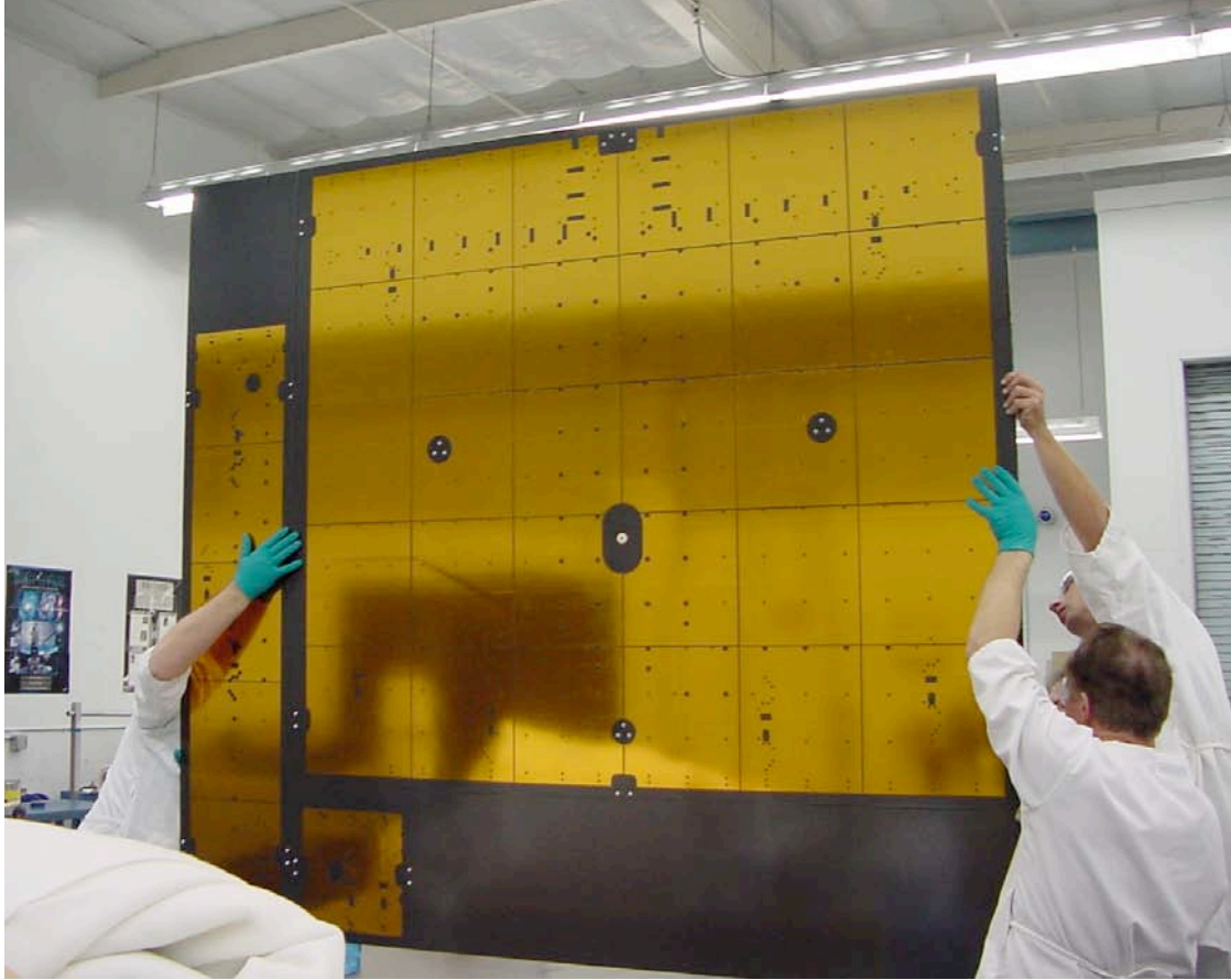
Figure 15. Photograph of as-cured flight substrate panel and qualification panels.
