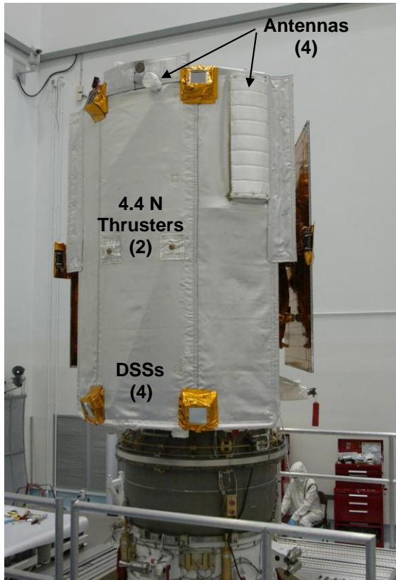
Figure 3. The MESSENGER spacecraft 2 weeks before launch. Highlighted here are the ceramic-cloth sunshade, the four digital Sun sensors (DSSs) with attenuating filters, the phased arrays and low-gain antennas under high-temperature radomes, and the 4.4-N pro-Sun thrusters.
