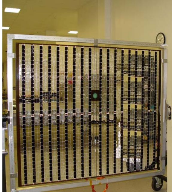
Figure 4. The MESSENGER +X solar array before spacecraft integration. Each solar array has a 2:1 ratio of OSRs to triple-junction gallium-arsenide solar cells.
