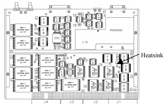
Figure 3: Backside of the MP and FPP Boards (the heatsink is used only for the MP Board)
