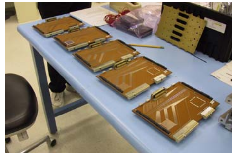
Figure 16: Dummy PWB Boards for the IEM Pre-engineering Vibration Test
