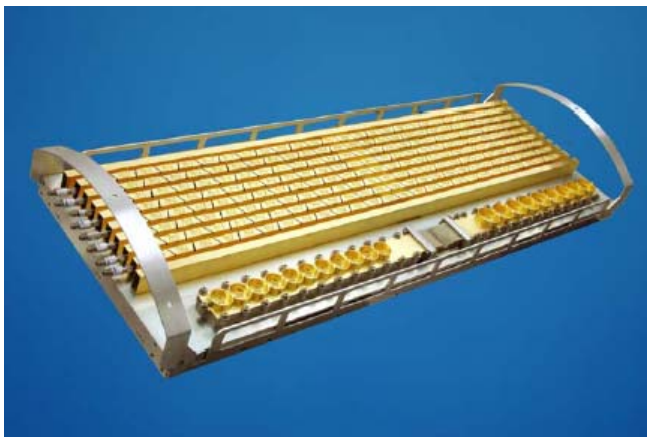
Figure 8. Phased-Array Antenna. It measures 11 inches by 32 inches.
