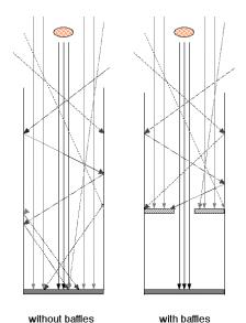
Figure 2. Without baffles, light from many directions enter the instruments and reach the detectors. By using the baffles, most of the stray light can be stopped from reaching the detectors.
