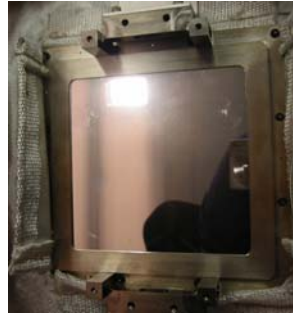
Looking through the ND filter as the DSS would (light source is a 1000w halogen lamp)
