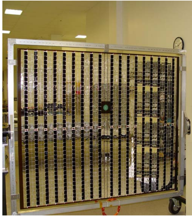
Figure 3. A MESSENGER solar array prior to integration. Illustrated here are the discrete strings of second-surface mirrors and solar cells
