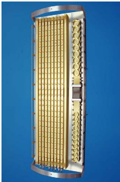
Figure 4. Flight phased-array assembly with radome removed. The fanbeam antenna is shown on the right
