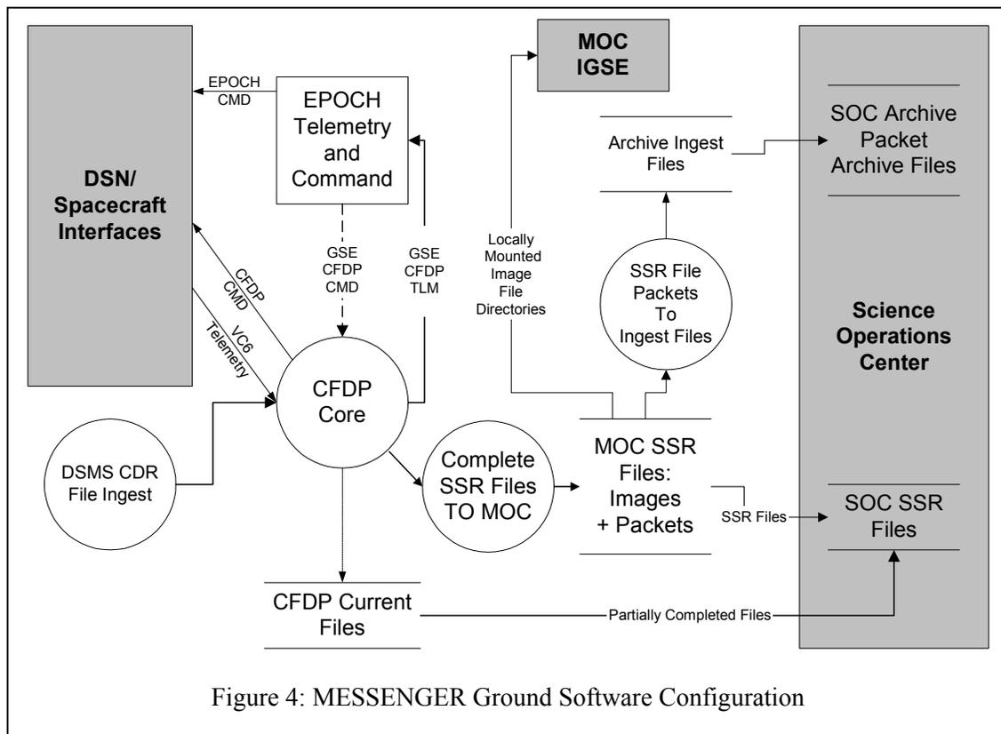
Figure 4: MESSENGER Ground Software Configuration
