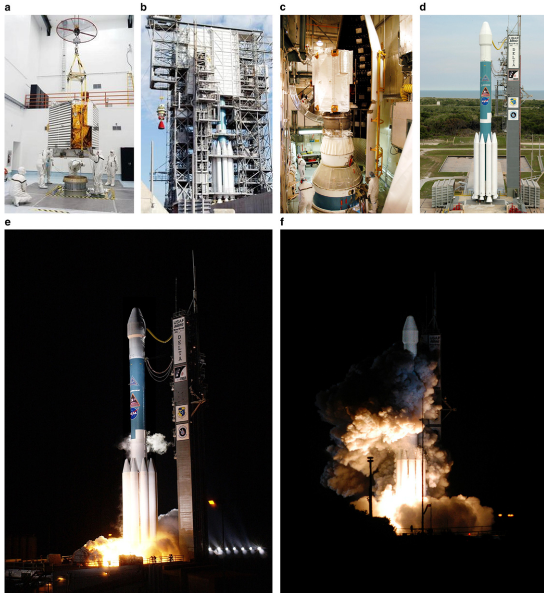
Fig. 3. Views of the MESSENGER spacecraft and launch vehicle from final testing through launch on 3 August 2004. (a) Spacecraft being lowered onto spin table (6 July 2004); (b) Delta II second stage being lifted up the mobile service tower (6 July 2004); (c) encapsulation of MESSENGER in shroud; (d) vehicle stack at Pad 17B (1 August 2004); (e) ignition; and (f) liftoff! (3 August 2004).
