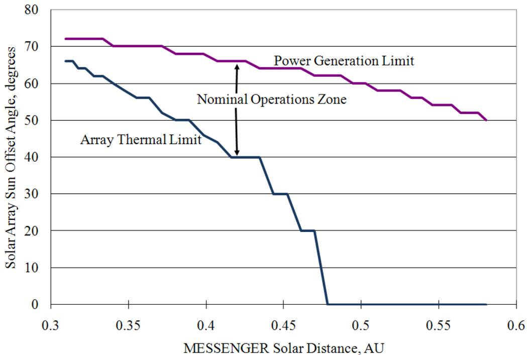
**Figure 3. MESSENGER Solar Array Sun-Offset Angle Limits**
