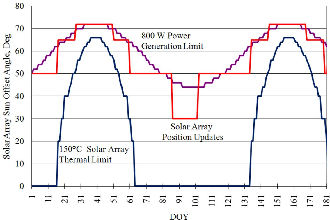
**Figure 4. MESSANGER Operational Solar Array Sun-Offset Angles for January – June 2009**
