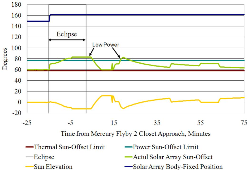
Figure 6. Actual Mercury Flyby 2 Solar Array Positions
