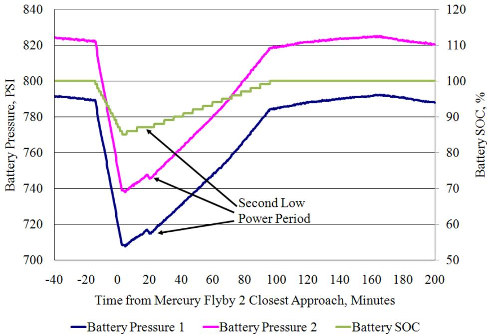
**Figure 8. MESSENGER Mercury Flyby 2 Battery State-of-Charge and Pressure**
