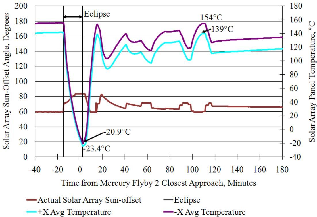
**Figure 7. MESSENGER Mercury Flyby 2 Solar Array Sun-Offset Angle and Panel Temperature**
