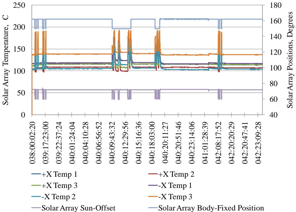
**Figure 9. Solar Array Position and Temperatures during the February 2009 Vulcanoid Survey**
