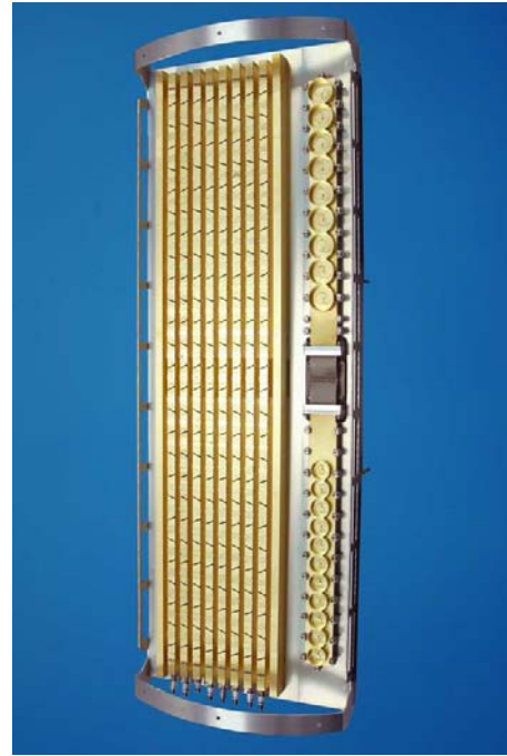
Figure 4. Flight phased array assembly with radome removed. The fanbeam antenna is shown on the right side of the assembly.
