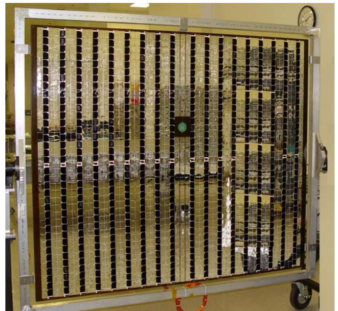
Figure 5. The MESSENGER +X solar array before spacecraft integration. Each solar array has a 2:1 ratio of OSRs to triple-junction gallium-arsenide solar cells.
