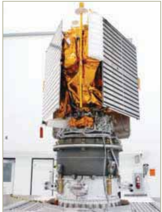
Fig. 6. The complex process of assembling and testing the MESSENGER spacecraft and mating it to its launch vehicle extended over a year and a half. Shown is the spacecraft on July 14, 2004, after it was attached to the payload assist module of the Delta II third stage at Astrotech Space Operations in Titusville, Florida. The two flat, reflective panels are the solar arrays stowed in their launch positions. (Image courtesy NASA and The Johns Hopkins University Applied Physics Laboratory.)
