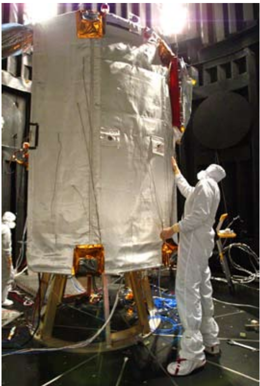
MESSENGER spacecraft during integration and testing. The sunshade is visible on the left with the spacecraft undergoing testing in thermal-vacuum conditions at NASA's Goddard Space Flight Center. On the right, the solar panels and Magnetometer boom are in their position for flight during work at APL.
