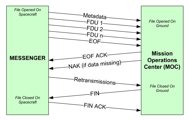
Figure 4 – Typical CFDP transaction provides reliable transmission of spacecraft file data
