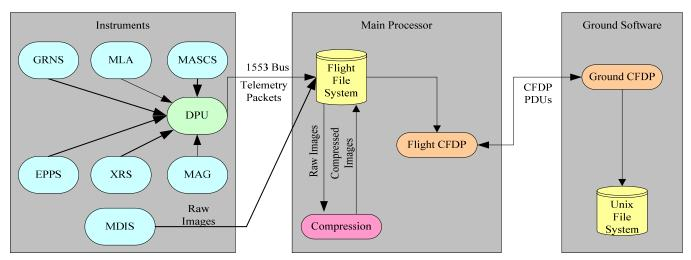
Figure 2 – MESSENGER instrument data flow with corresponding mirrored CFDP and file storage
