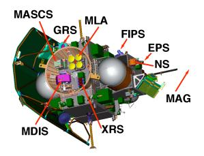
**Figure 9**: The directional instruments (MDIS, MASCS, MLA, and XRS) are mounted inside the launch vehicle adapter ring.
