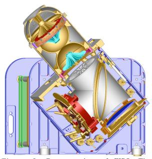
**Figure 8**: Cutaway view of FIPS. The electrostatic analyzer is at the top and the time-of-flight section extends to the lower right.
