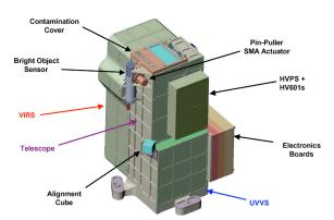
**Figure 6**: MASCS combines surface and exospheric observations in a small instrument.
