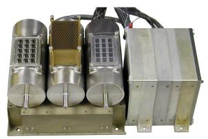
**Figure 4:** Engineering model of the planet-viewing portion of XRS.
