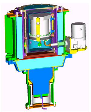
Figure 2: Gamma-ray spectrometer.
