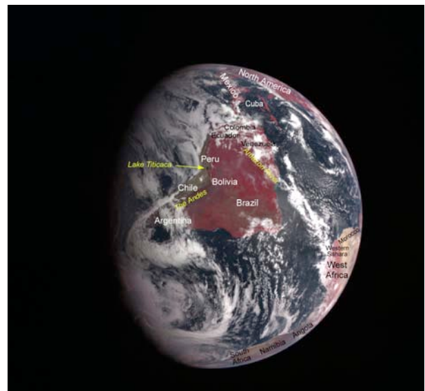
Fig. 7. A false-color image acquired with three exposures using three different filters on the wide-angle camera component of MDIS.
