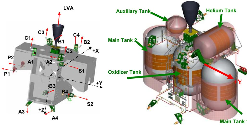
**Figure 2. MESSENGER Thrust Directions and Tank Layout**
