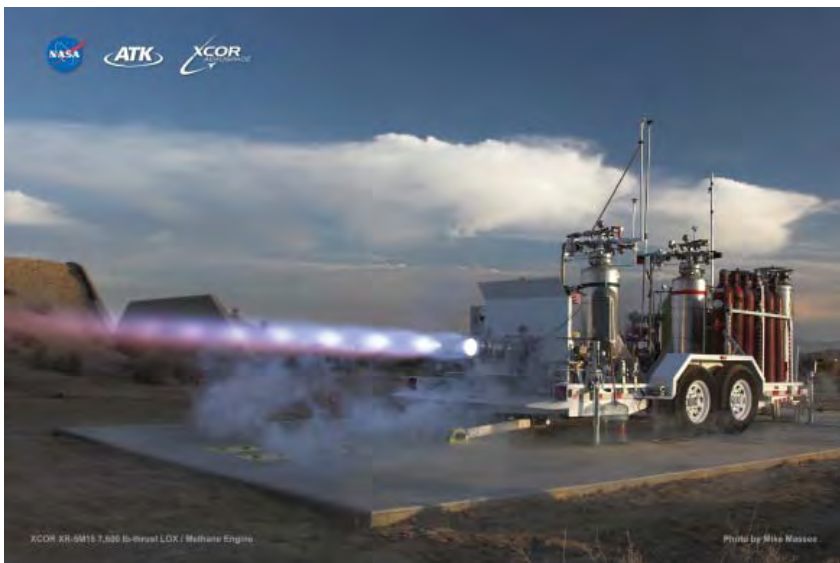
Figure 1. Test fire of the XR-5M15 Trombone Engine on the 40K test stand.
