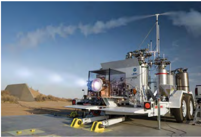
Figure 2. A test fire of the XR-5M15 Workhorse Engine at XCOR's Mojave test facilities.
