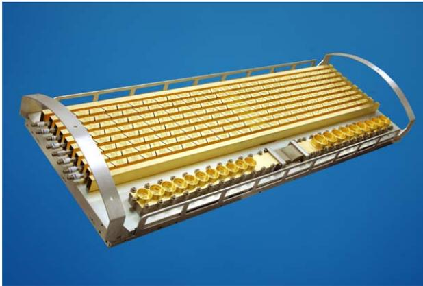
**Figure 2 Flight Phased-Array and Fanbeam Antenna Assembly**
